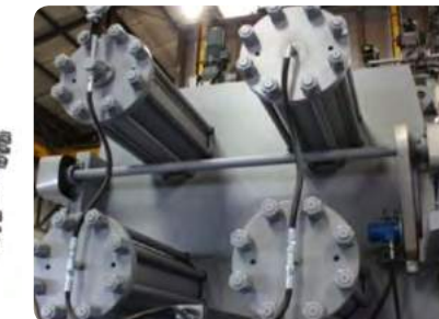
· 4-Head Hydraulic Cylinder Structure
